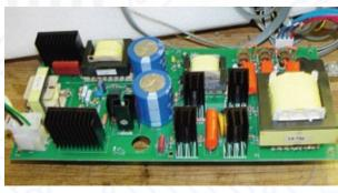
Diagnostic LEDs on both remote diagnostic PCB, and main ballast board, and also dry contact for sensing, and alarming both ballast/lamp operation, and failure.
