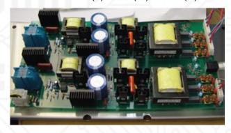
Diagnostic LEDs on both remote diagnostic PCB, and main board, and also dry contact for sensing, and alarming both ballast/lamp operation, and failure.
