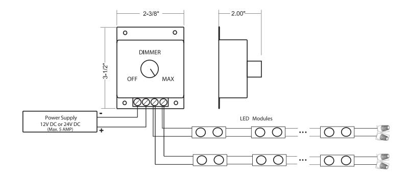
\*Allanson LED Dimmer (PWM) will dim all 12V and 24V LED Modules, except for the 1 Watt (ACLW-CW-1W) and 3 Watt (ACLW-CW-3W) modules, and the LED Saber.
