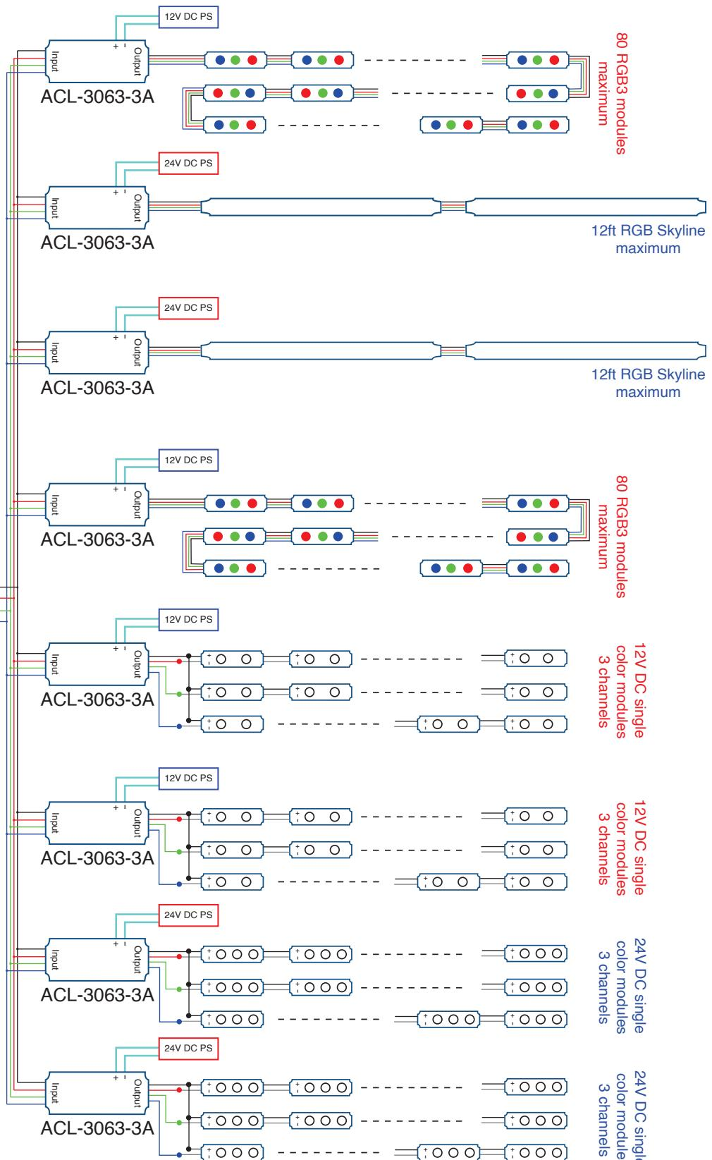
12V lamp connected, loads 0~60W(12V)
