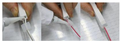
5. Place end cap on tube and seal with silicone (wait 10 minutes)
