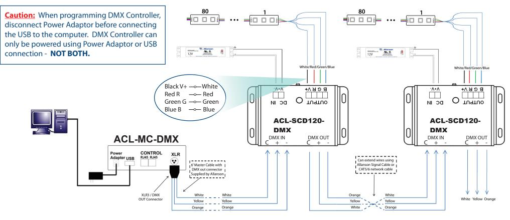
Each Allanson 60W Power Supply (CV125 series) can run maximum 80 ACLW-RGB3 modules.
